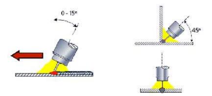
When welding with flux-cored wires, move the welding gun in pulling angle to prevent the slag generated by the wire from mixing with the molten weld. The arc pressure will keep the slag behind the molten weld. Certain directional welds, such as upward welding, are an exception to this. In this case the welding gun is moved with the handle behind the direction of movement, and earth's gravity ensures that the slag will not rise above the molten weld.
